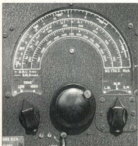
Fig. 5: Tuning scale on the PCR, showing the locking feature immediately below the tuning knob (see text).
